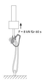
The braking device is fastened with the additional attachment to the testing equipment. The rope is attached using a 10 mm pin. A force of 8 kN is applied to the rope for 60 seconds.
