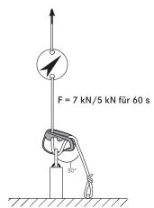
In the case of a single rope (twin rope: 7 kN two strands, half ropes: 5 kN one strand) a force of 7 kN must be applied to the braking device for 60 seconds.
